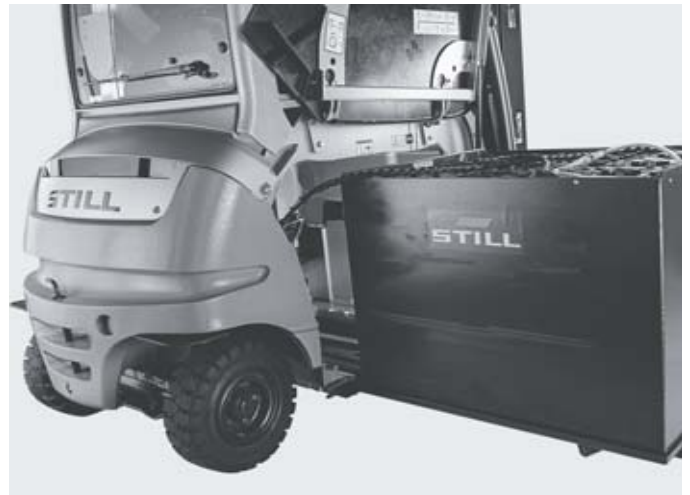
Battery replacement system (option)
