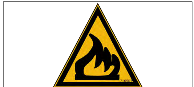
Figure 29: Autocollant - Danger Liquides inflammables
